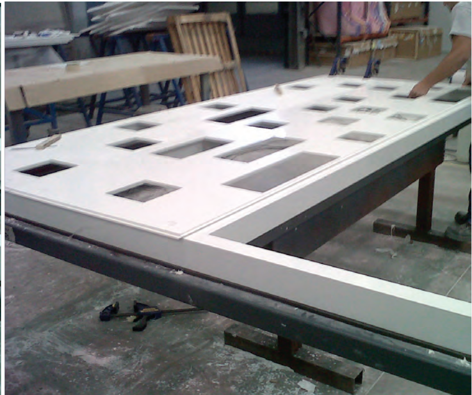
INSTALLATION OF MECHANIZED KRION® SHEETS
