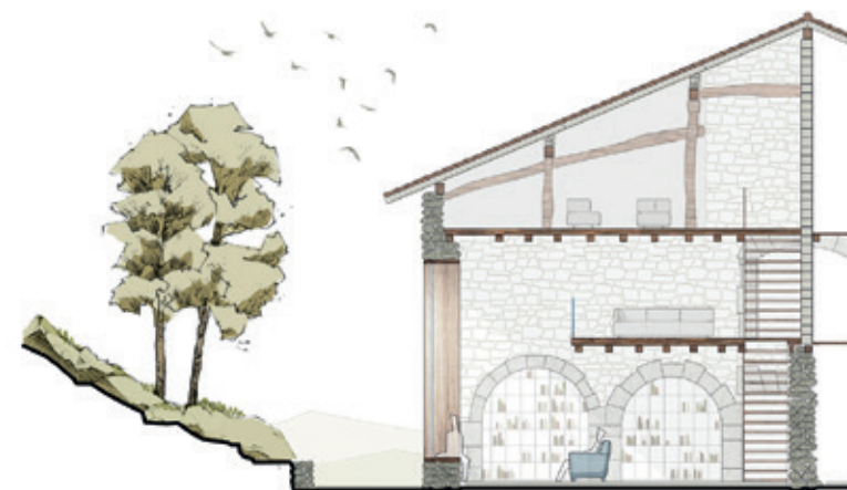
A modern staircase was created to connect the ground floor – the new living area – with the first floor, where the bedrooms are. The top floor, once the house's original drying room, is now an open-plan space. The Bilbao Architecture Team studio reinforced the original stone and oak structure, and at the same time, made it visually lighter by installing PAR-KER® Steel Oxford ceramic parquet by Porcelanosa and other ceramic flooring by Venis .
